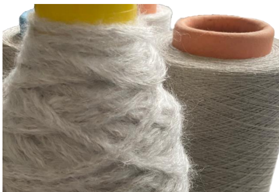
Figure 1 Air Flow and Single yarns made from hemp and Lyohemp®
