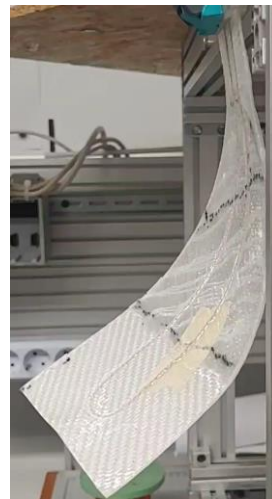
Figure 1 Example of an integrated fibre rubber composite structure subjected to bend-twist coupling
