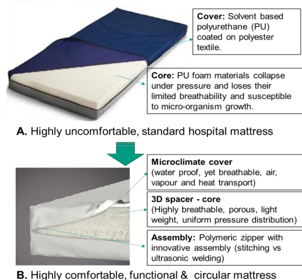
Figure 1 Proposed circular (mono-material) and functional mattress (B) and its comparison with standard mattress (A).
