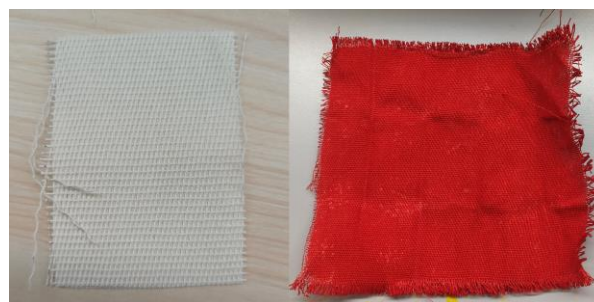
Figure 1 Paper-based knitted fabric before and after dyeing
