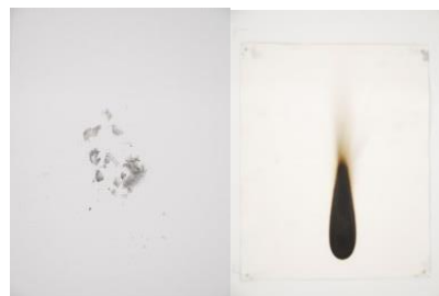
Figure 1 Cotton after flame test according to ISO 15025, without flame-retardant finishing (left) and finished with phytic acid/chitosan.
