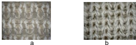
Figure 1 Photos of knitted fabrics: a – Sample B; b – Sample C The tensile properties of knitted fabrics were measured by KES-F (Kawabata Evaluation System), Tensile and Shear Tester (KES-F-1). The parameters obtained for tensile hysteresis curves are defined in Table 1.
