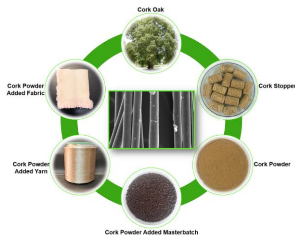
Figure 1 Production cycle of cork powder added polyester yarn
