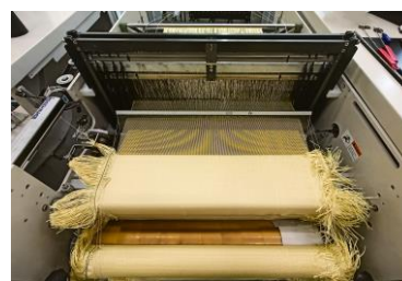
Figure 2 Rapier weaving machine CCI with dobby shedding mechanism.
