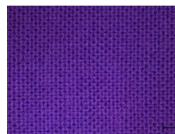
Figure 1 Cotton fabric dye with Methylene Blue and Rose Bengal
