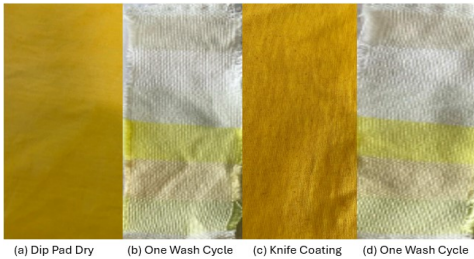
Figure 3 (a) Impregnated by dip-pad-dry (b) Impregnated by dip-pad-dry after one wash (c) Coated by knife coating (d) Coated by knife coating after one wash.
